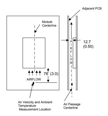
Wind Tunnel Test Setup Figure
